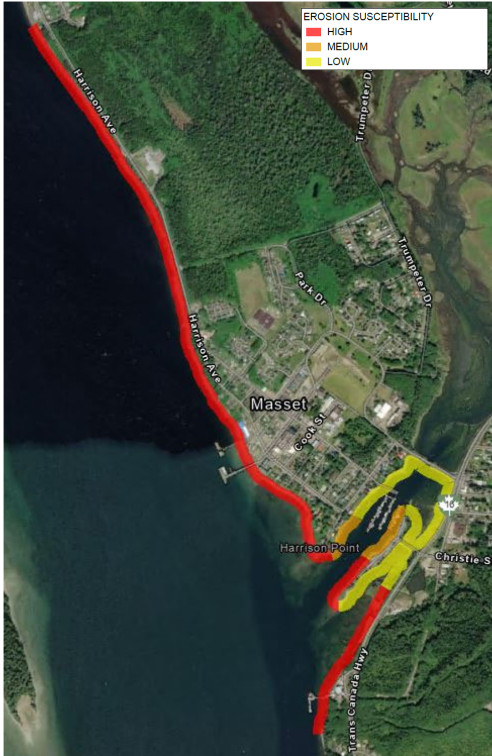
Figure 3-1. Portion of map of erosion susceptibility for the southern portion of the Village of Masset study area.
